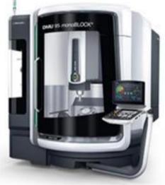
DMG MORI 5 Axis CNC Milling Center DMU95
