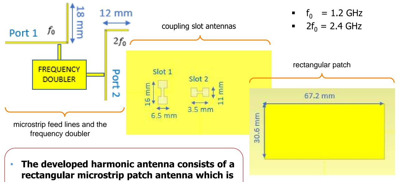
fed with two orthogonal microstrip lines coupled with the patch through H-slots
